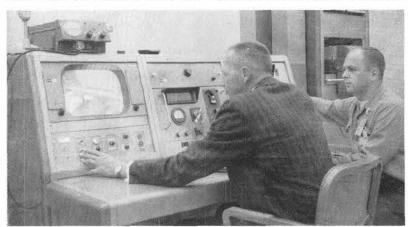
TELEVISED IMAGE of arrow rocket on monitor screen in console building at Sandia's Hot Gas Facility is adjusted by E. J. Meyer, left, and D. R. MacKenzie (both 7132-1). The facility uses rocket engines to produce gas jets for aerodynamics experiments.
